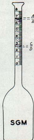
Fig. 14. Milk tests are read from the base of the lower meniscus to and including the upper meniscus, or from A to D as shown in the diagram.
