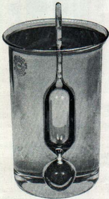
Fig. 5. Testing acid for strength by means of the acidometer.
