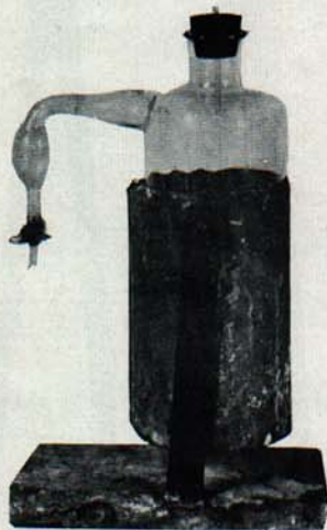
Fig. 8. Acid bottle which automatically measures 17.5 cc. of acid.
