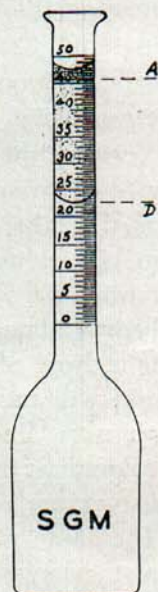
Fig. 17. Cream sample showing how glymol will break the top meniscus. The sample is properly read from the base of the lower meniscus to the line formed by the glymol and butterfat, that is, from "A" to "D".
