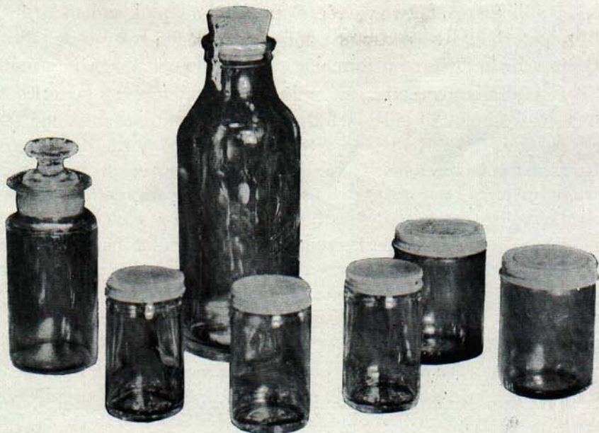
Fig. 3. Three-ounce screw-top sample jars are best for cream samples; rubber-stoppered jars for milk composites.
