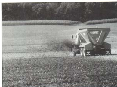
Side-delivery spreaders can apply solid biosolids very uniformly when using the surface application method.
