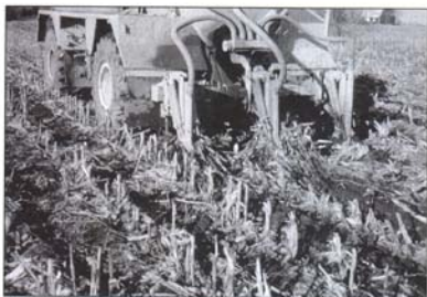
Applying liquid biosolids from the West Bay County TWTDs to cropland by injection into the soil.
