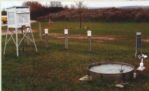
A weather station and an evaporation pan generate data for pest management and irrigation decisions.
