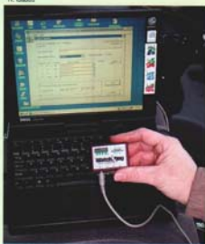
A laptop computer downloads weather data collected at a fruit farm for pest monitoring.
