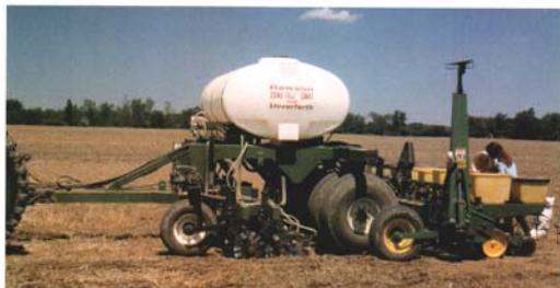
22-inch zone-till equipment with corn planter.
