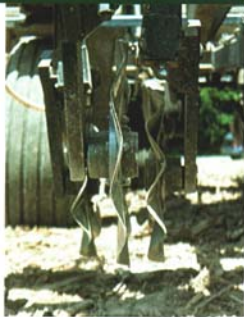
Close up of 3-coulters zone-till system.
