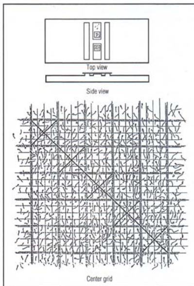
Figure 6. Diagram of both top and side views of a hemacytometer, and the center grid area where sperm are counted in order to estimate sperm concentration.
