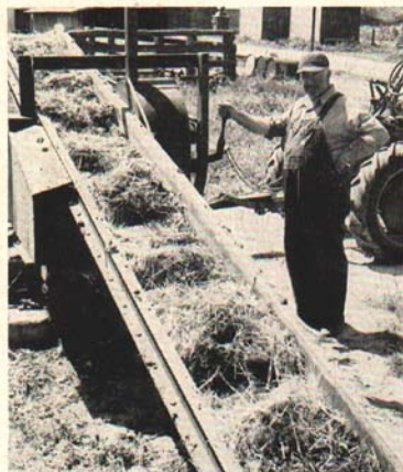
Fig. 3. Note strong foundations. The unit is anchored in cement. Mr. Cable of Bath, Michigan, is holding the clutch handle. The power unit and winding drum are located above the base.
