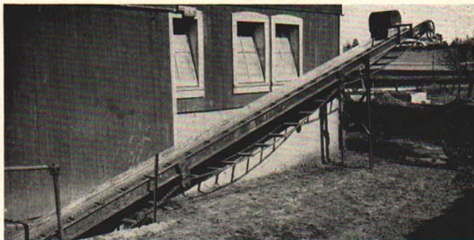
Fig. 16. The loading elevator on the Brook Brothers farm, Haslett, Michigan. This type is used on the double-gutter dairy barn in which an endless apron cleans the gutter and drops the manure onto the lower end of the loading elevator.
