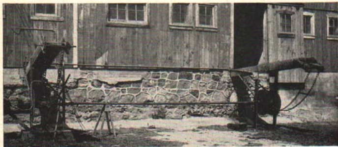
Fig. 7. Power, clutch and shaft arrangement of a dairy barn where one motor and a gear reduction unit operate both aprons of a two-gutter, face-in-type barn. The clutches are grab type. (George Bailey farm in Hillsdale County.)
