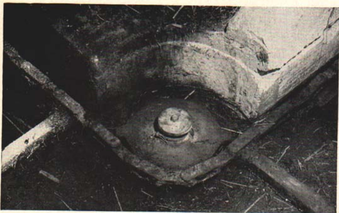
Fig. 20. Corner idler. Note chain construction and steel rail in bottom of gutter which takes all wear.
