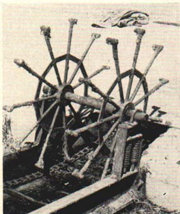
Fig. 2. Spider-wheel. Note the well braced construction and spring tensions. The wheel holds down the apron as it starts up the loading chute.
