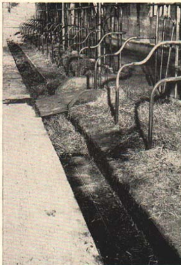
Fig. 5. The interior view of the A. J. Cable dairy barn, showing the single gutter and the return cable on the lower end. Note how clean the gutter is left as the apron moves out.
