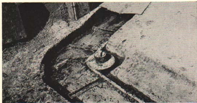
Fig. 15. Tightener idler. This idler is on an eccentric hub which is used in tightening the apron chain.
