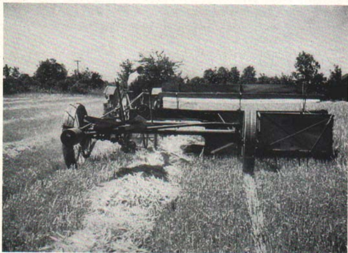
Fig. 3. Cutting and windrowing barley with a windrowing machine.
