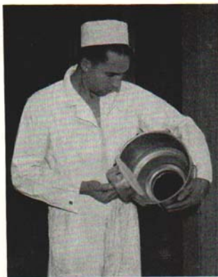
Fig. 9. An excellent kind of strainer is being assembled for use. The pad is ready to be inserted. The flow of milk from the pail does not fall directly onto the pad.
