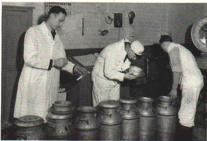
Fig. 1. A final check on milk quality is the tests made at the "platform" when milk is delivered. At left, the inspector takes the samples for his tests. The men who weigh and empty the cans also take tests and examine the milk for flavor.
