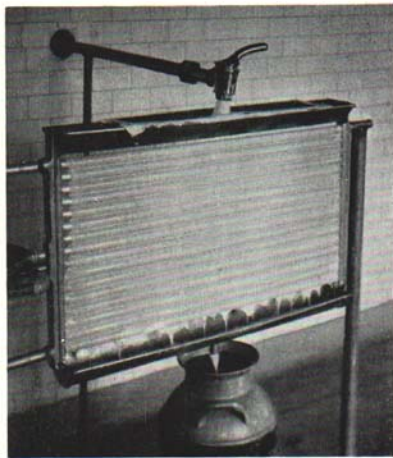
Fig. 8. A tubular cooler with the milk coming from the strainer tank in adjoining room and being rapidly cooled to 40° F.
