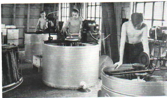
Fig. 28. Extracting equipment. Note "wing" comb supports in first extractor. Note arrangement, comb tables near each extractor, honey piped through floor, motors mounted above extractors with V-belts, ample room to truck empty supers on platforms away from extractors.
