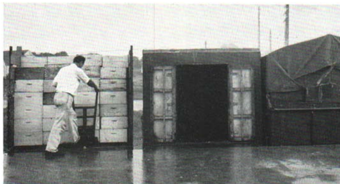
Fig. 25. An unloading dock saves much labor. A rubber-wheeled warehouse truck is used to load and unload supers.
