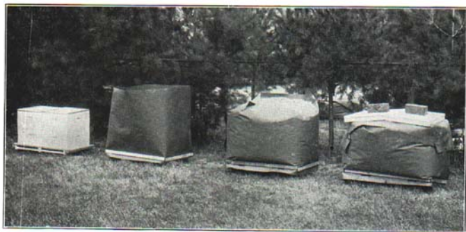
Fig. 41. The four steps in preparing the asphalt-paper packing-case, using loose packing on sides and top.
