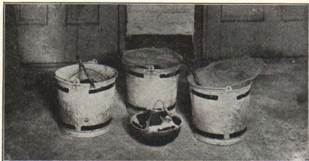
Fig. 1. Equipment used in fumigating with sulphur.
