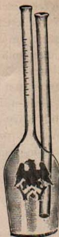
FIG. 18. A skim-milk test bottle on which each subdivision represents .05 of one percent.
