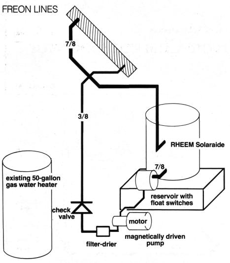
Fig. 2 An active system charged with Freon-114.
