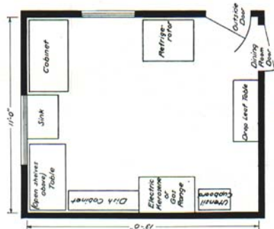
Fig. 30. A broken U-arrangement using portable equipment.
