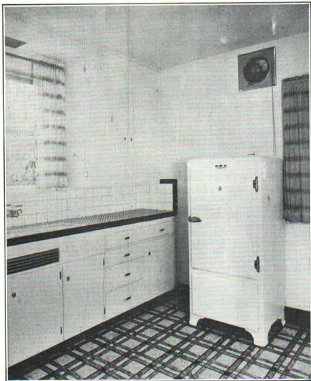
Fig. 1. The two windows provide adequate light and cross-ventilation. The electric fan in the wall above the refrigerator quickly rids the kitchen of undesirable odors. (Another view of the kitchen in Fig. 18.)
