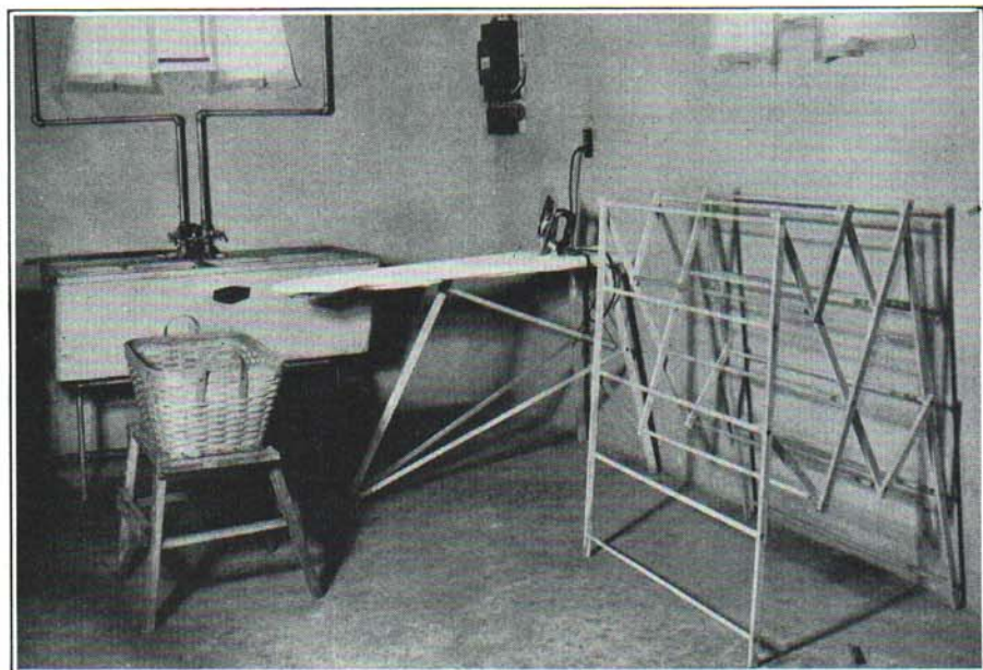
Fig. 3. The washing center of Fig. 2 converted into an ironing center. Note the following: portable ironing board with removable cover, outlet for iron cord, stand for basket, clothes bars. The high windows provide good light and ventilation.
