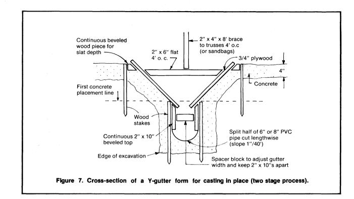
Fresh concrete should be vibrated to fill the space beneath the inner frame, to prevent water leakage from the gutter, and to provide a smooth surface. A semicircular bottom can be constructed by cutting a 6- or 8in. PVC pipe in half lengthwise and nailing the half-pipe in the bottom of the inner frame.
