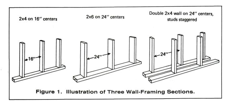
16 in. or 24 in. centers is becoming more popular in an attempt to approach "superinsulation" while still using more or less standard framing techniques. Finally, double-wall framing is sometimes used, with potential R values of 40 and more (see Figure 1). Other, more exotic, superinsulation techniques have been successful, but generally result in high labor or material costs and questionable return on investment.
