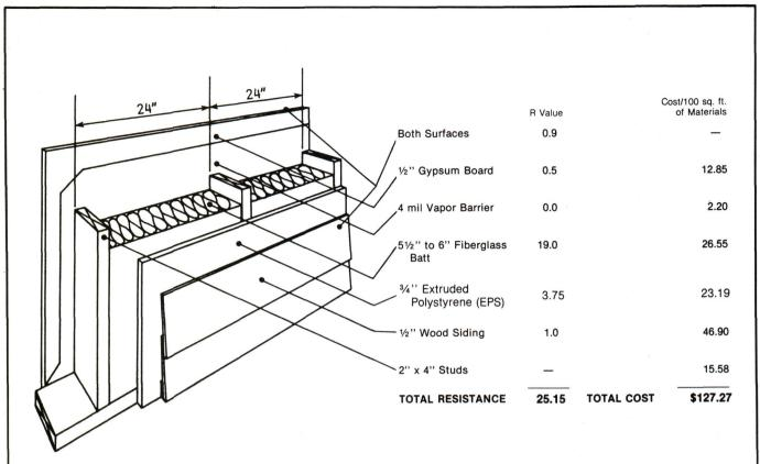
Figure 4. A 2 x 6 Framing Technique with EPS.
