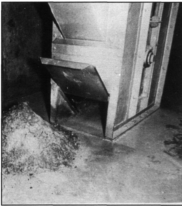
Figure 4. Elevator legs can hold sizable amounts of residual feeds or ingredients. Some of this material can be incorporated in the next batch of feed.
