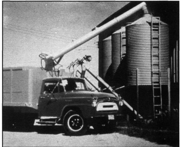
Figure 6. A feed delivery truck can be a source of drug carry-over. Feed can remain in the lower horizontal conveyor and in the vertical conveyor. Although the amount of residual feed depends on the design of a particular system, residual feed can range up to 100 pounds.
