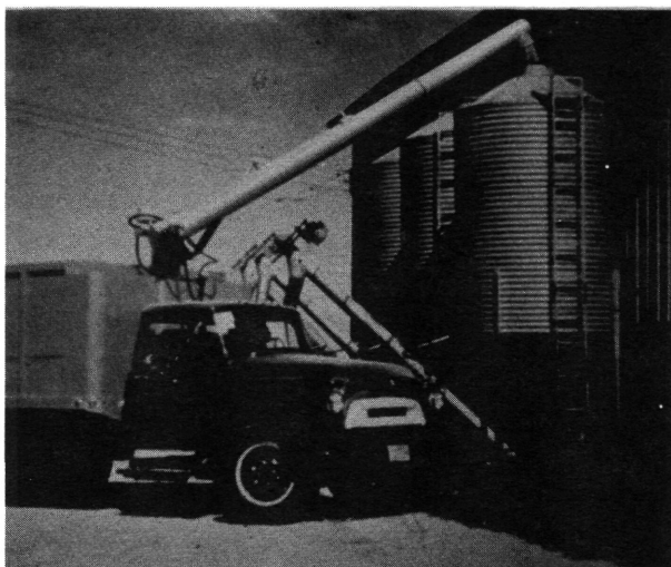
Figure 6. A feed delivery truck can be a source of drug carry-over. Feed can remain in the lower horizontal conveyor and in the vertical conveyor. Although the amount of residual feed depends on the design of a particular system, residual feed can range up to 100 pounds.
