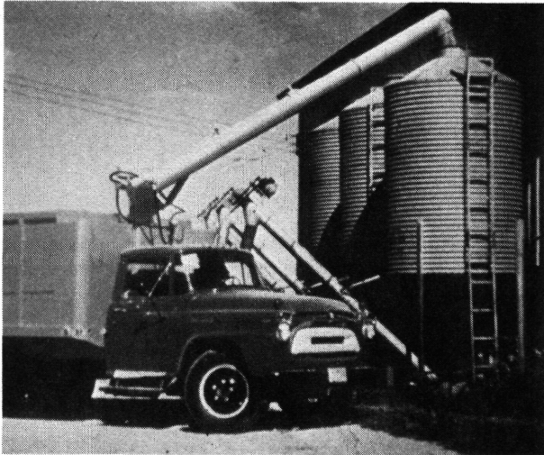
Figure 5. A feed delivery truck can be a source of carry-over. Feed can remain in the lower horizontal conveyor and in the vertical conveyor. Although the amount of residual feed depends on the design of a particular system, residual feed can range up to 100 pounds.
