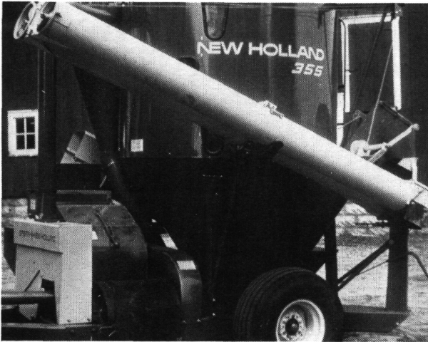
Figure 1. This type of grinder-mixer is commonly used on hog farms. Mixers can harbor excessive residual feed and dust, and must be cleaned after mixing sulfa-medicated feed.
