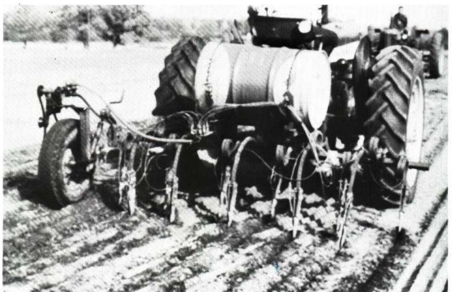
Figure 10. Injection of soil fumigant using a shank-type applicator.
