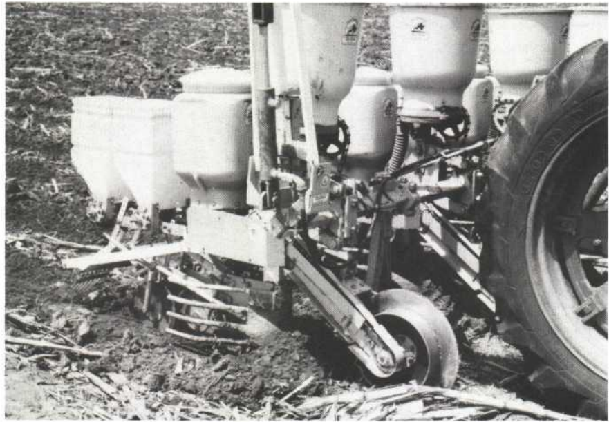
FIGURE 3. Buffalo All-Flex Till Planter with dry fertilizer, seed, insecticide and herbicide hoppers, depth control disk, and trash guards. The sweep that clears a planting area is below and in front of the trash guards. A 10-inch zero pressure seed press wheel firms seed into moist soil. Photo — Fleischer Mfg., Inc., Columbus, NE
