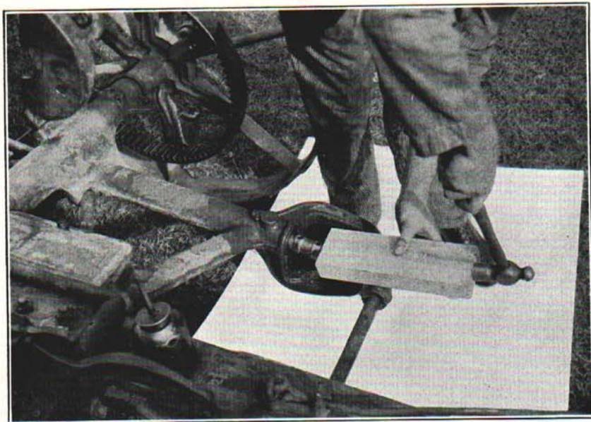
Fig. 7. Replacing lower crankshaft bearing. Fly-wheel removed.
