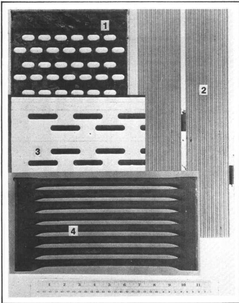
**Figure 6. Flooring materials that have been used in nurseries.**
