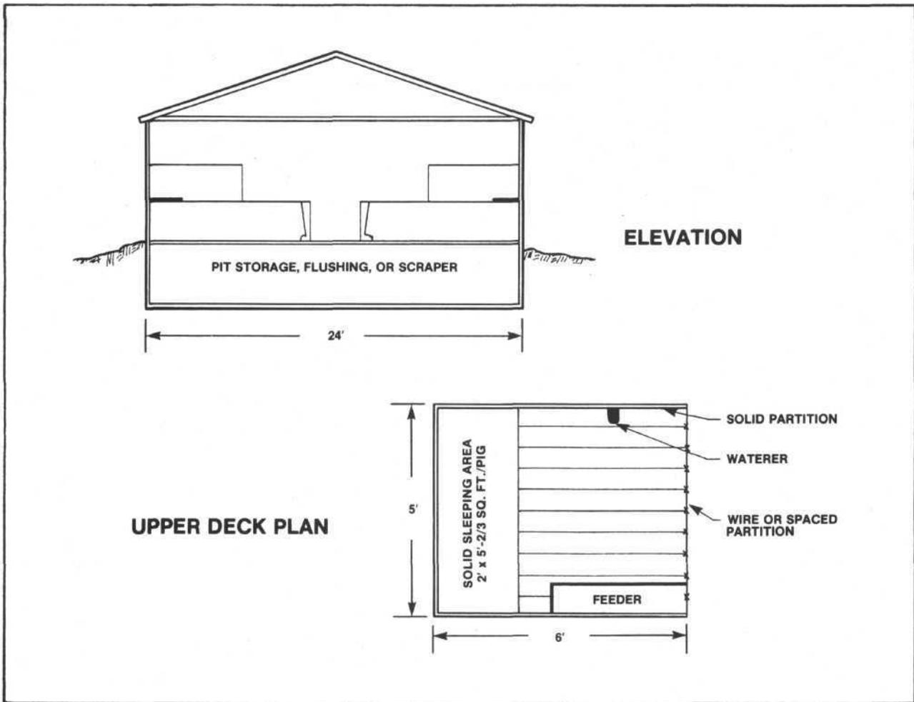
**Figure 2. Views of decked nurseries which were added over existing nursery pens. An alternate arrangement for the top pens would be to locate the sleeping area and feeder in the front near the aisle and the waterer in the rear of the pen over the slotted floor.**
