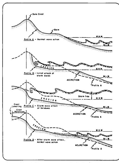
Figure 12. Schematic diagram of storm wave attack on beach and dune.
