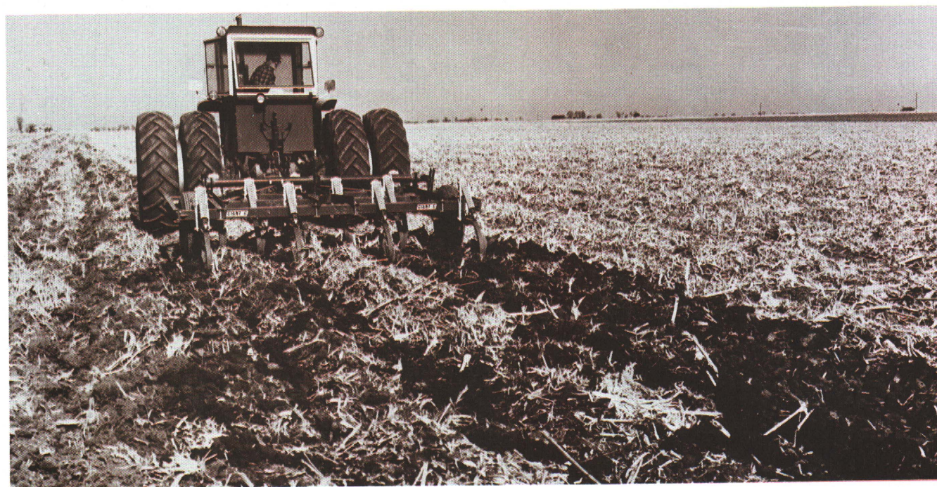
Figure 4. Chisel plows should be large enough and strong enough to penetrate compacted soil. The curved chisel shovels generally leave less crop residues on the surface than do the narrower standard straight shovels. A coulter in front of each chisel would help to prevent plugging with corn stalks.
