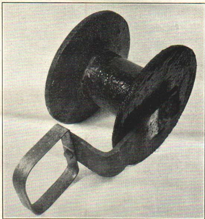
Fig. 10.—The roller used in moving the hose.
