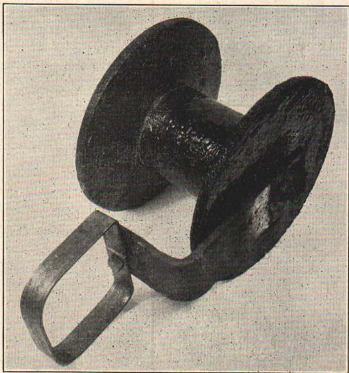
Fig. 10.—The roller used in moving the hose.
