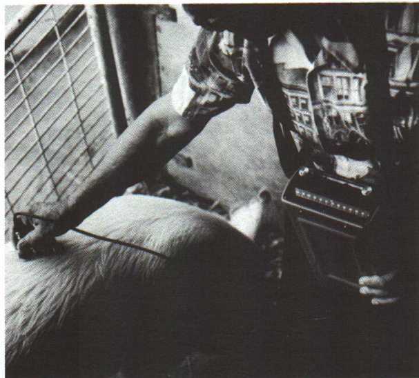
Figure 4b. Ultrasonically measuring for backfat thickness.
