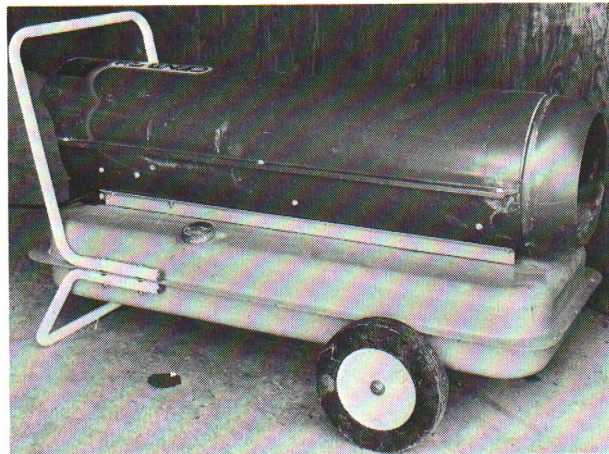
Figure 3. Temporary-type portable heater using fuel oil as the energy source. Blower and controls connect to 115 volt outlet.
