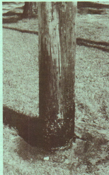
Fig. 8. Bleeding poles like this result in preservative loss from upper parts but service life is probably not decreased if not moved. If used as a spring pile some surface oil on water could result.
