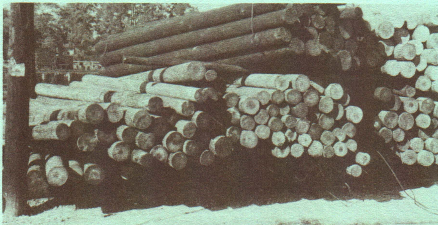
Fig. 4. Color variation in pine posts treated with PCP in oil.
