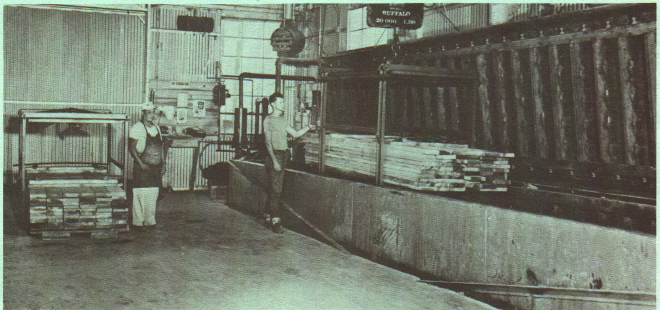
Fig. 5. Treating lumber with PCP water repellent solution by vacuum process. Tank cover will be closed and vacuum drawn on lumber. (Photo courtesy of Robert's Consolidated Industries.)
