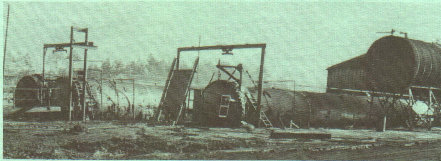
Fig. 7. Three treating cylinders used for full cell or empty cell pressure treating.
