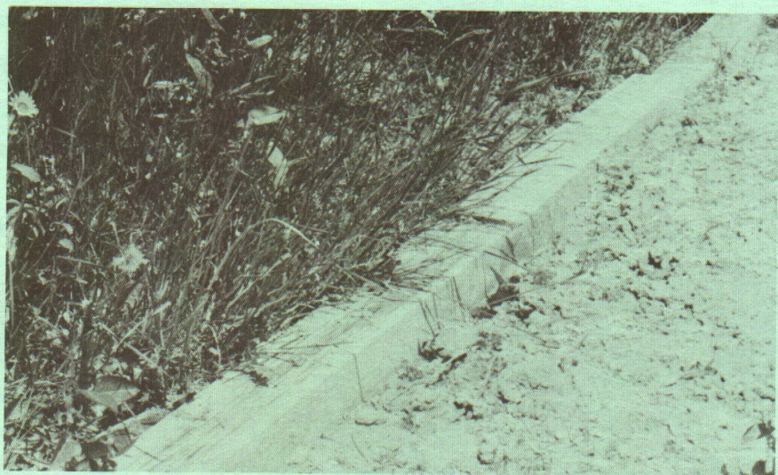
Fig. 5. Grasses growing adjacent to wood pressure-treated with 5% PCP solution in oil.
