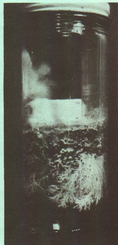
Figs. 3a and b. Soil block toxicity test on wood preservative. Treated blocks are placed in jars of soil with growing decay fungus.
