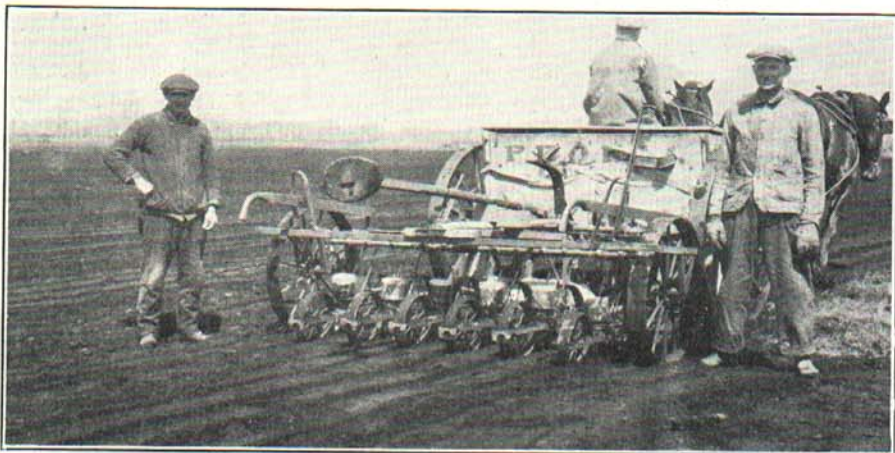
Fig. 6. A combination fertilizer drill and onion seeder. Six rows are sown with the fertilizer applied in the row below the seed by the fertilizer drill ahead. Just behind the drill, a light float smooths the surface of the muck ahead of the seeders. In some cases a garden tractor is used to sow three rows, the row fertilization and seeding generally being done in separate operations. On the larger farms nine-row and twelve-row outfits, tractor drawn, have additional seeders attached to sow a row of barley between every three rows of onions for wind protection.
