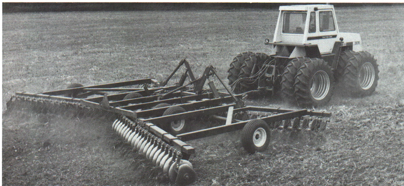
Figure 4—The disc loosens the surface soil to a depth of several inches but compacts the soil immediately below tillage depth. Opportunities for excessive compactness increase with soil moisture levels. It is seldom that the disc loosens the soil to the depth of compaction caused by the tractor pulling the disc.
