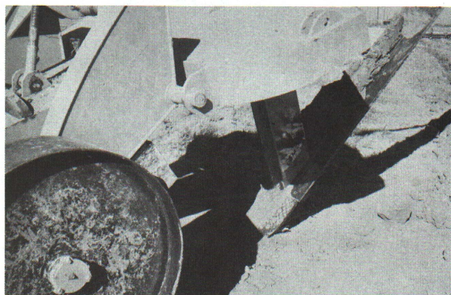
Figure 2-B—This single tooth chisel subsoiler is designed for deep penetration. The "foot" has a lifting action which is effective only when used on dry soil. Deep subsoiling should not be attempted on wet soil.
