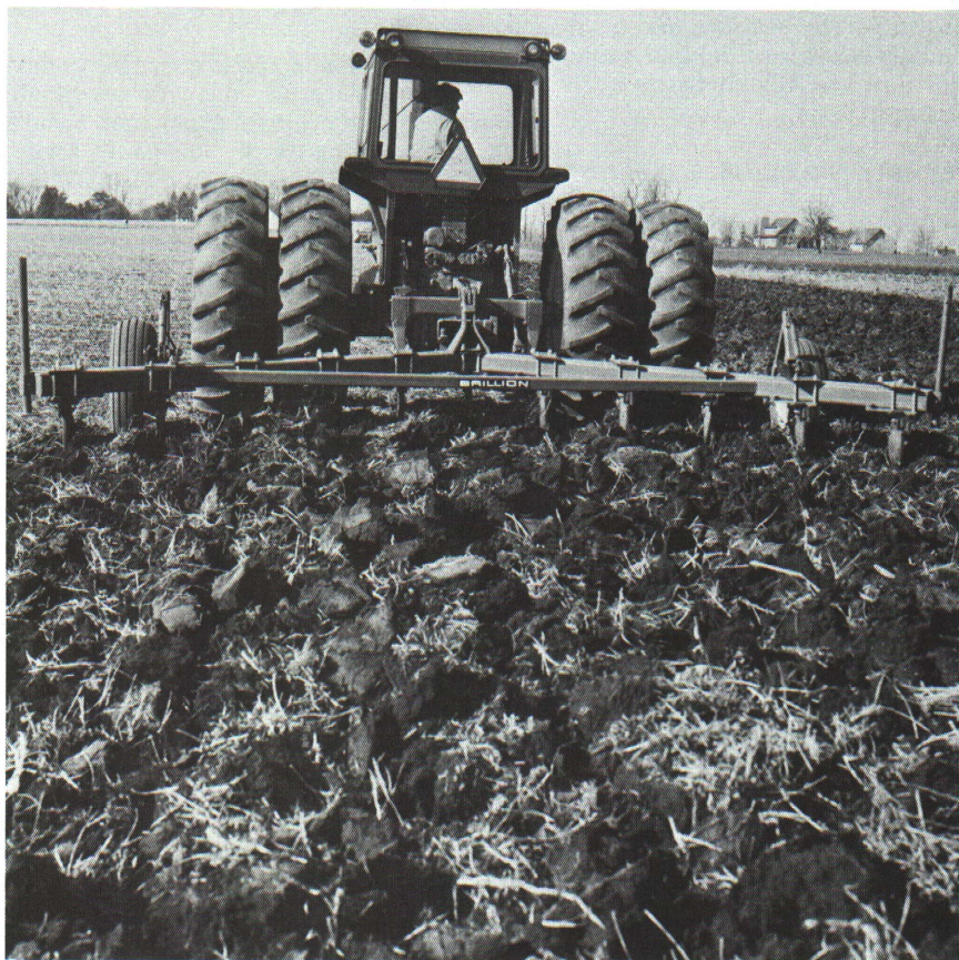
Figure 3—Modern multiple-shanked subsoiler. The tillage effect is more complete than with single-shank shown in Figure 2. Depth of penetration frequently is limited with multiple-shank tools. Such implements are especially well suited for destroying tillage pans or for loosening relatively shallow compact horizons.
