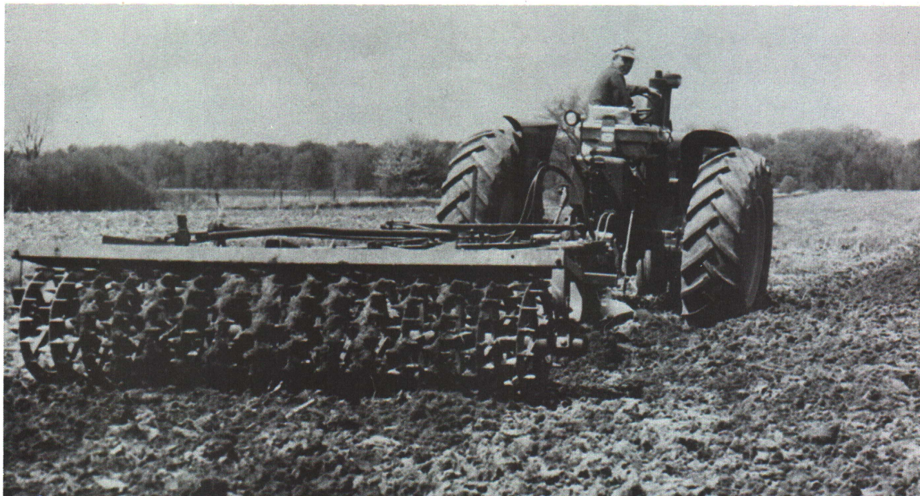
Figure 12—Trailing minimum-tillage tool. This was once a popular soil treatment in Michigan but is now used less extensively because many feel that it is difficult to transport from one field to another. Used behind a plow, it firms the surface soil and easily breaks down clods, thus reducing the need for secondary tillage. Where secondary tillage can be eliminated, earlier planting is possible.
