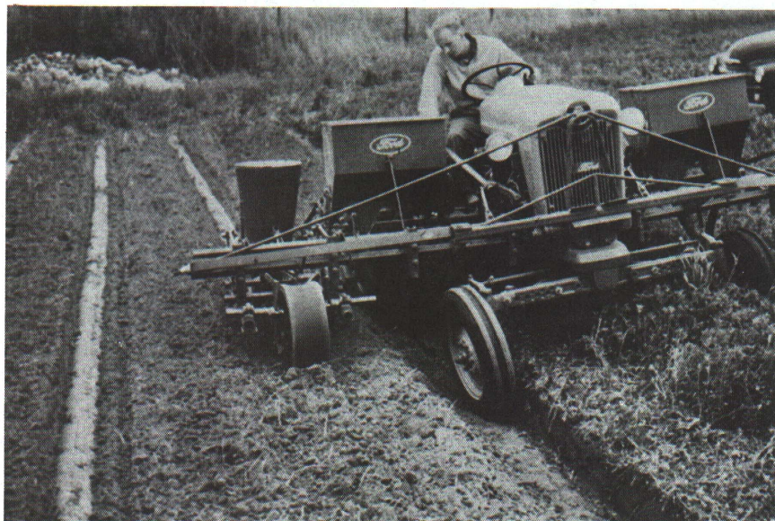
Figure 7—Moldboard plowing and planting in one operation with research implements. The soil between the rows contains in excess of 40% air space, which retards weed seed germination. It is in good condition to receive and store water from a heavy rain. The ideal moisture level for plowing is also the ideal level for rapid seed germination. Press wheels on the planter firms moist soil around the seed, insuring rapid germination. A well-adjusted plow on this well-drained medium-textured soil is loosening the soil and greatly improving its porosity.
