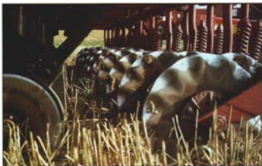
Fluted coulters need to be adjusted for downward pressure for proper zone tillage.
