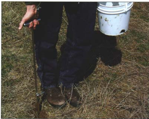
Collect soil cores with a sampling device like this step-in soil probe.
