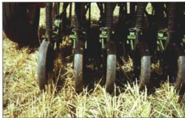
Adjust downward pressure of press wheels for good soil-seed contact.
