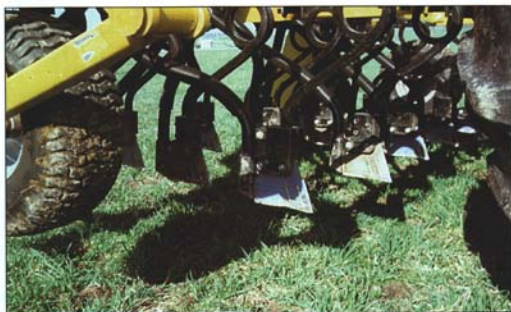
A no-till drill with coil tine and sod-slicing Baker Boot opener without a disc couler used in overseeding pastures.
