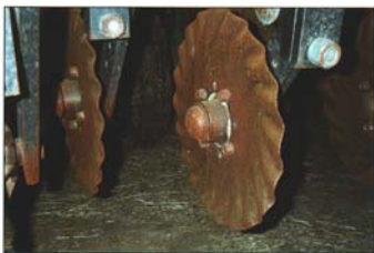
Fluted coulters are used for cutting through crop residue.
