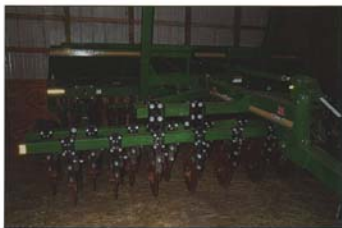
A no-till drill with fluted coulters for ease in cutting through crop residue.
